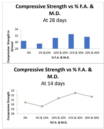
The accompanying graph shows that the maximum comp. strength is reached with 15% fly ash and 30% marble dust. The maximum amount is 15% fly ash and 30% marble dust. The optimal percentage of fly ash and marble dust is reached, and as the percentage of fly ash and marble dust increases, the composite strength steadily decreases.
