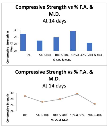
The graph above shows that the maximum composite strength is reached with 15% fly ash and 30% marble dust. The maximum amount is 15% fly ash and 30% marble dust. The optimal percentage of fly ash and marble dust is reached, and as the percentage of fly ash and marble dust increases, the composite strength steadily decreases.
