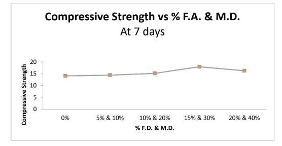
The accompanying graph shows that the maximum compressive strength is reached with 15% fly ash and 30% marble dust. The maximum amount is 15% fly ash and 30% marble dust. As the percentage of fly ash and marble dust increases, the compressive strength steadily decreases.
